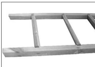
2 Lay the notched framework on a flat surface. Slide in the three identical steps as far as they will go into each notched section of both frames. Screw each step into place using 2x 60mm screw, 1 at each side.
