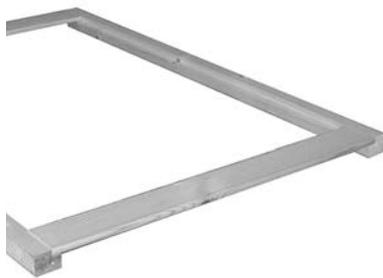
1 Place the two rebated sections on a firm level surface. Place on the rebated section two of the slats – one at either end of the rebate. Drill and screw into place using 2x 25 mm screws per slat, one at either end.
