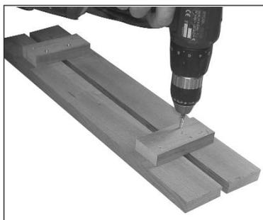
1. Place two pieces of shutter side by side, the edge to edge measurement should be approx 115 mm. Place one block in the centre of two shutter pieces screw approx 75 mm from the top and fix using 4x 25 mm screws in each block, two screws into each shutter piece. Place a further block at the bottom and fix as previously described. Repeat.
