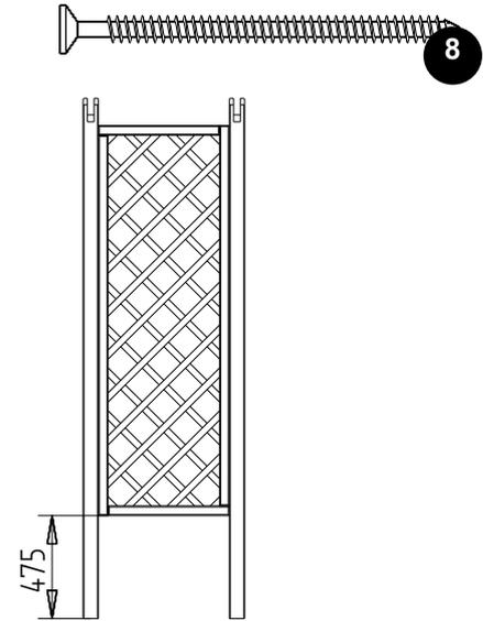
If you are not using a post support system it is recommended that you locate the posts 30cm into the ground.
