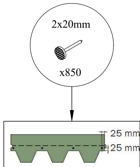
**Carefull ! The shingle overlay must be about 134 mm.**
