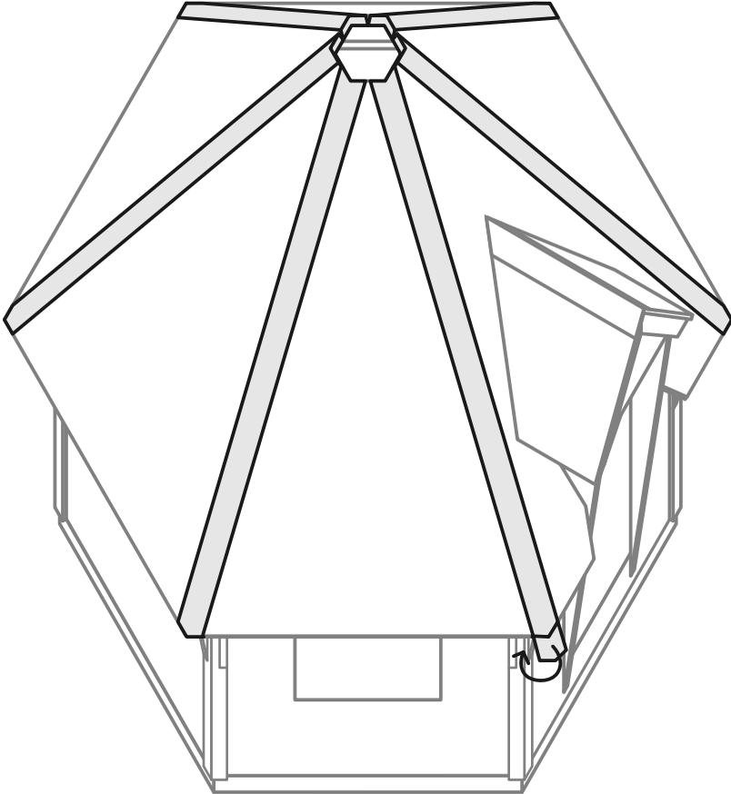
Attach peak plates to the connecting brims of the roof elements. Use felt nails. The lowest plate should be placed 7cm over the lower brim, flipped under the eaves and secured with nails.
