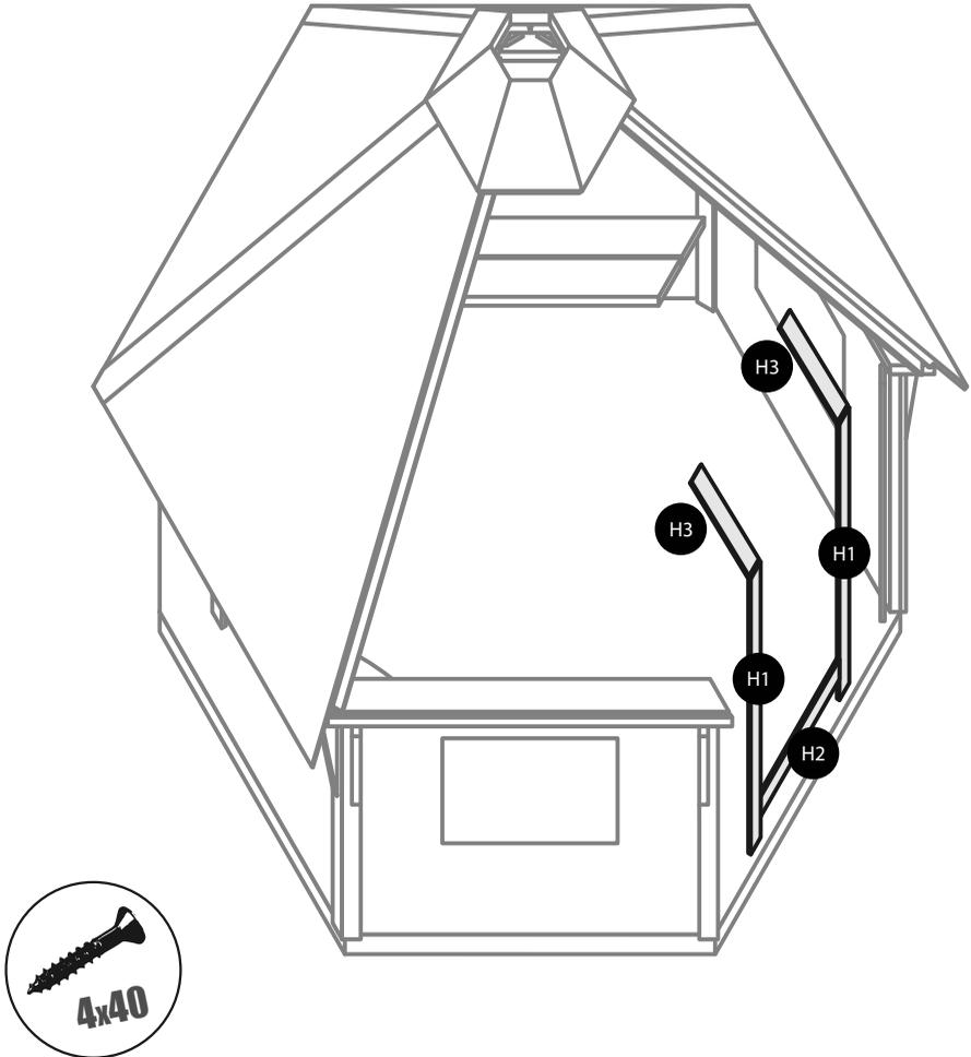
Attach door strips inside the grillhouse. The strips are attached to the door frame, wall element and roof element with 3 screws per detail.
