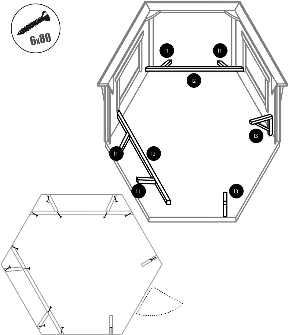
Attach the bench beams by first attaching the longer detail to the wall elements from the ends. Make sure they are parallel to the wall. Then attach the two shorter details to the previously attached detail and to the wall. Beams should be placed 39cm above the floor.
