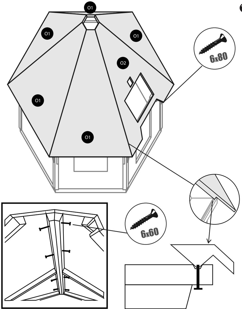
Be sure to provide support for each roof element while assembling. Use 8 screws to attach wall elements to one another and another 4 from under the brim planks. Make sure when placing the roof element with door hole (O2) that the gaps are even to the wall element's.
