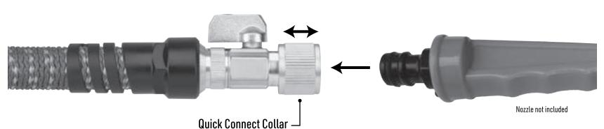
Pull back the spring loaded collar to both disconnect and connect hose guns and nozzles
